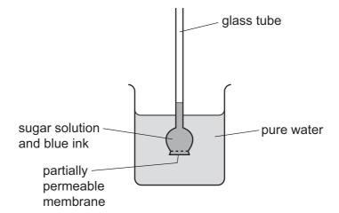
Some hours later, the water in the beaker had turned blue, and the liquid in the glass tube had moved upwards.
